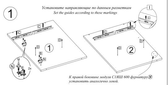
To the right sidewall of the module T1DB 600, install the accessories the same way as the left sidewall.
